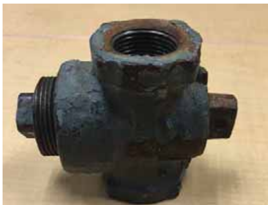
Figure 2: Typical 3/4" Nordstrom Service Valve
