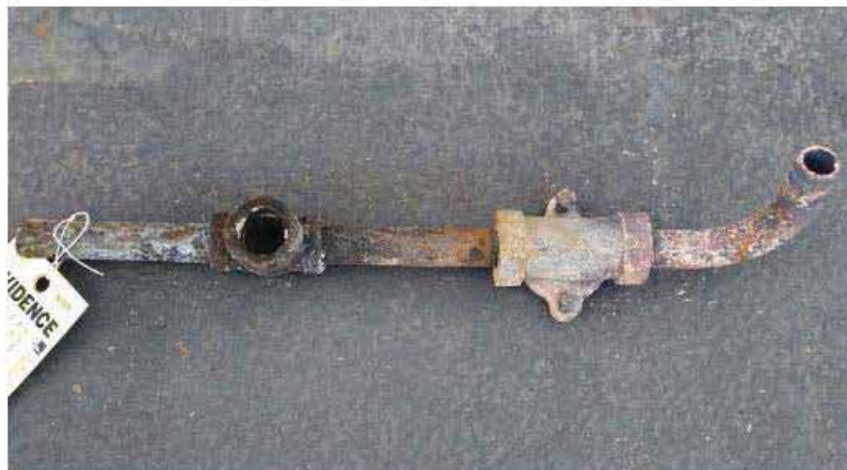
Figure 1. As found service valve body and piping.
