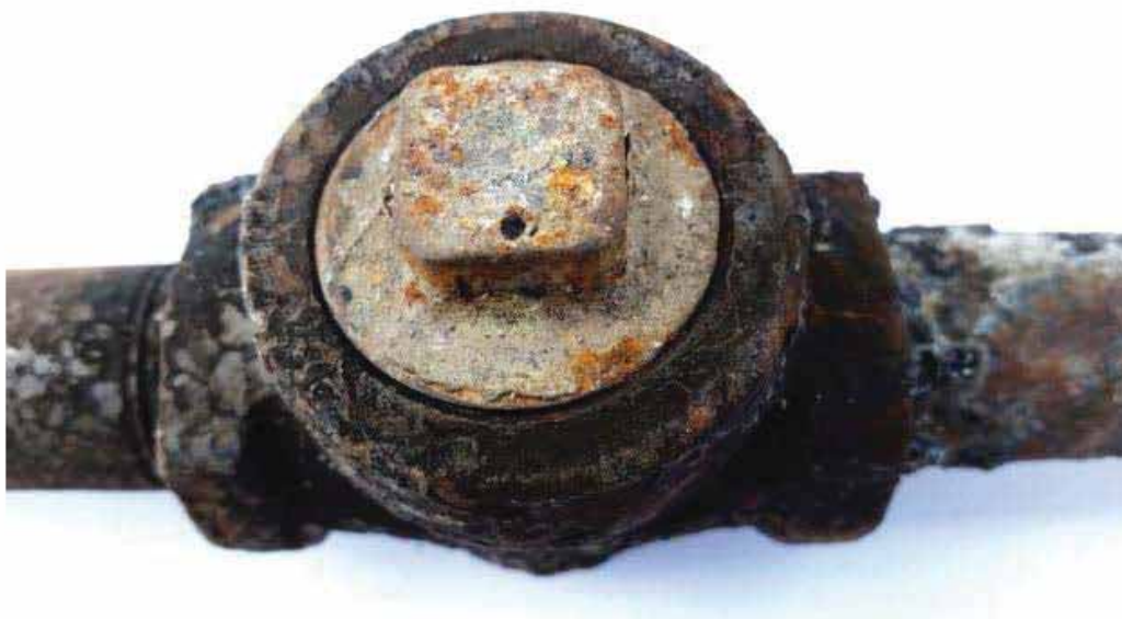
Figure 10. Square head plug level to the top surface of the valve body.
