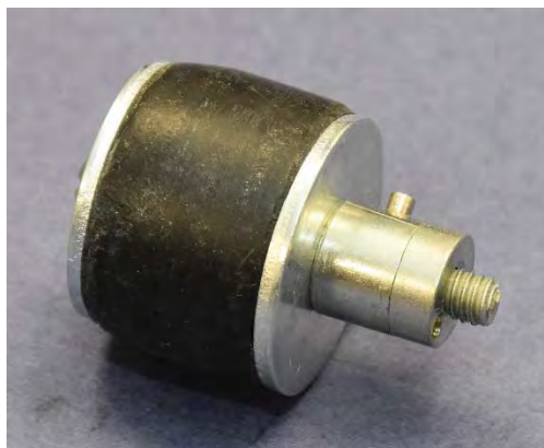
Figure 37. X-Pander plug in an unexpanded state.
