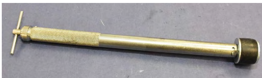
Figure 38. X-Pander plug mounted on an installation tool.
