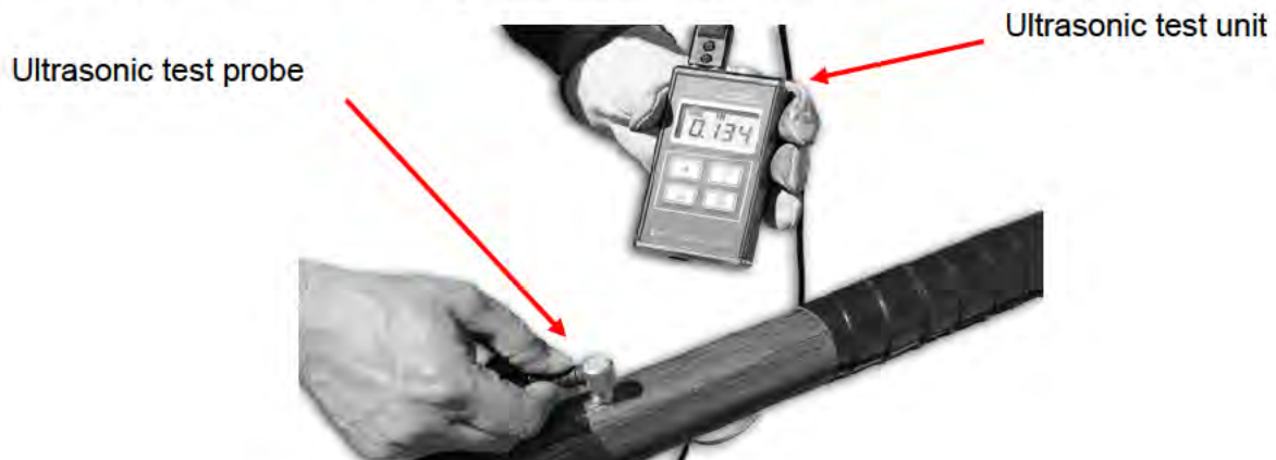
Figure 1. Check Pipeline Wall Thickness
