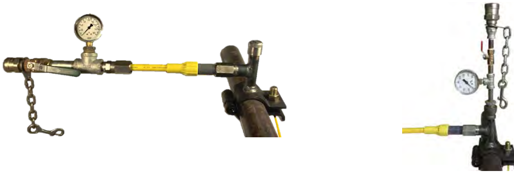
Figure 6. Typical Pressure Test Assembly Installed
