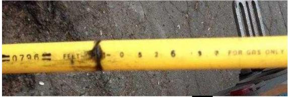
Figure 6: Date stamp on inserted plastic for service of indicating 052697. Failure Analysis
