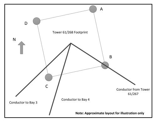
Figure 2: Tower Foundation Layout and Conductor Location
