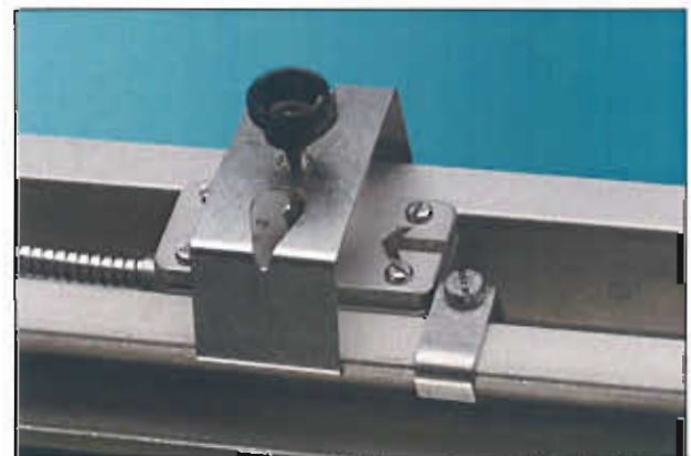
M2N transducers in the Variotix rail
