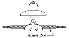
FIGURE 15-9: ARMOR RODS USED WITH SUSPENSION INSULATORS
