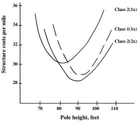
FIGURE 13-2: STRUCTURE COST PER MILE RELATED TO POLE HEIGHT
