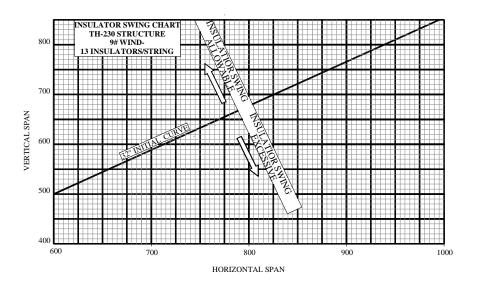
FIGURE 7-3: TYPICAL INSULATOR SWING CHART FOR A TH-230 TANGENT STRUCTURE (Moderate Wind Swing Condition Only, 9 psf assumed instead of minimum NESC 6 psf, No Line Angle Assumed)
