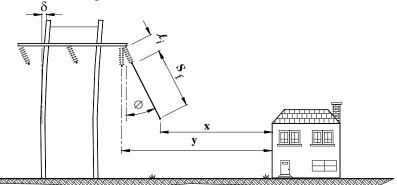
FIGURE 5-1: HORIZONTAL CLEARANCE REQUIREMENT TO BUILDINGS
