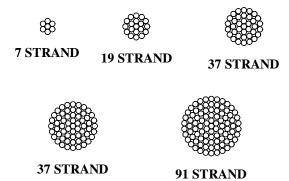
FIGURE 9-2: 1350 ALUMINUM CONDUCTOR STRANDINGS
