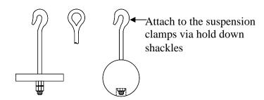
FIGURE 15-13: DISC WEIGHTS (Left), BALL WEIGHTS (Right)
