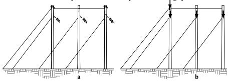
FIGURE 14-5: AXIAL LOADS INDUCED IN A POLE
