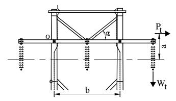
FIGURE 13-17: POLE TOP ASSEMBLY WITH INSIDE BRACES
