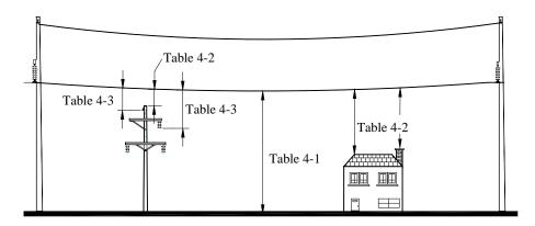
FIGURE 4-1: CLEARANCE SITUATIONS COVERED IN THIS CHAPTER
