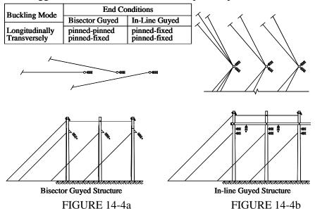
FIGURE 14-4: END CONDITIONS FOR BISECTOR AND IN-LINE GUYED STRUCTURES
