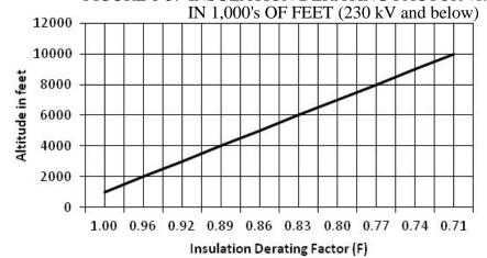
Curve is a plot of the equation: F= (17.93B)/(460 + T) Where T = 60° F and B is standard atmospheric pressure at various altitudes in inches of Hg.
