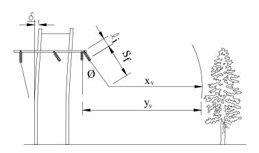
FIGURE 5-2: RADIAL CLEARANCE REQUIREMENT TO VEGETATION
