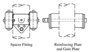
FIGURE 15-17: SPACER FITTING, REINFORCING PLATE AND GAIN PLATE
