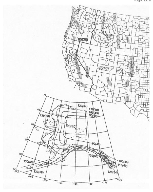
FIGURE 11-2a: BASIC WIND SPEED IN MILES PER HOUR AT 33 FT. ABOVE GROUND For use in calculating Extreme Wind Load (50-year mean recurrence interval). From IEEE C2-2012, National Electric Safety Code® (NESC®), Copyright IEEE 2012. All rights reserved.
