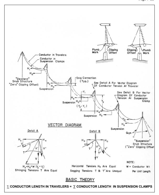
FIGURE 9-7: ANALYSIS FOR APPLICATION OF CLIPPING OFFSETS From IEEE Standard 524-2003, "IEEE Guide to the Installation of Overhead Transmission Line Conductors," copyright 2004 IEEE. All rights reserved.
