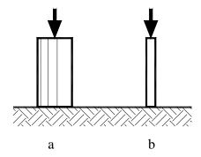
FIGURE 14-2: COMPARISON OF RODS TO SHOW STABILITY CONCEPT
