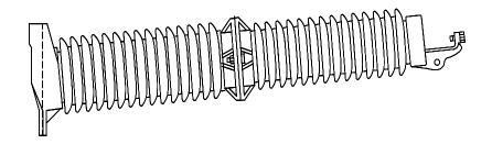
FIGURE 8-2: A TYPICAL CERAMIC HORIZONTAL POST INSULATOR
