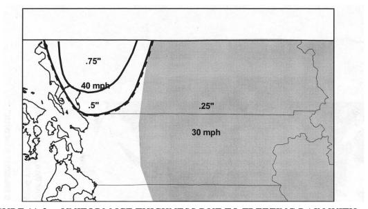
FIGURE 11-3e: UNIFORM ICE THICKNESS DUE TO FREEZING RAIN WITH CONCURRENT 3-SECOND GUST WIND SPEEDS FOR FRASER VALLEY DETAIL (50 yr. mean recurrence)
