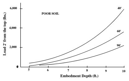
FIGURE 12-1: EMBEDMENT DEPTHS IN POOR SOIL
