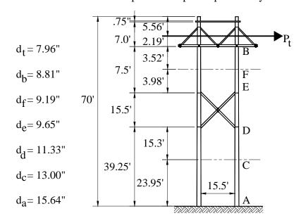
FIGURE 13-24: EXAMPLE OF AN H-FRAME
