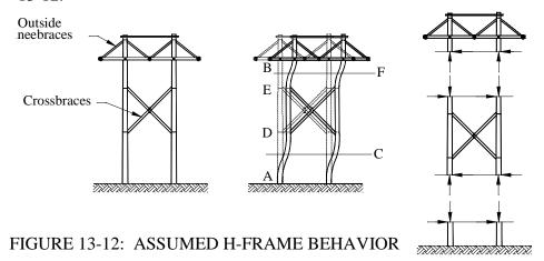
At some point in the poles, there will be an inflection point (a point of zero moment). If the pole or column is uniform in cross section, it is common to assume that the inflection point is located midway between points of bracing, shown as a dotted line in Figure 13-12. However, since the pole is tapered, the following relationship may be used to determine the location of the inflection point (see Figure 13-13, Equation 13-16 and Appendix H for application chart).
