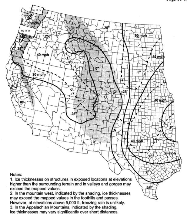
FIGURE 11-3a: UNIFORM ICE THICKNESS DUE TO FREEZING RAIN WITH CONCURRENT 3-SECOND GUST WIND SPEEDS (50 yr. mean recurrence)
