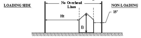
FIGURE 5-7: SIMPLIFIED RECOMMENDATIONS FOR CLEARANCES TO GRAIN BINS WITH PORTABLE LOADING EQUIPMENT Total Horizontal Clearance = Ht = (24' + B) + 1.5B Horizontal clearance is for highest voltage of 230kV
