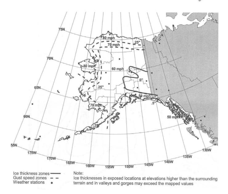
FIGURE 11-3c: UNIFORM ICE THICKNESS DUE TO FREEZING RAIN WITH CONCURRENT 3-SECOND GUST WIND SPEEDS FOR ALASKA
