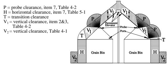
FIGURE 5-3: CLEARANCE TO GRAIN BINS NESC FIGURE 234-4a From IEEE C2-2012, National Electric Safety Code® (NESC®), Copyright IEEE 2012. All rights reserved.
