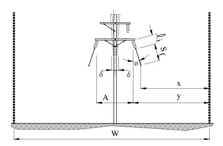
FIGURE 5-9: ROW WIDTH FOR SINGLE LINE OF STRUCTURES
