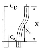
FIGURE 13-13: LOCATION OF POINT OF CONTRAFLEXURE
