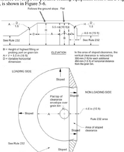
The clearance envelope for portable loading equipment from NESC Figure 234(b), is shown in Figure 5-6.
