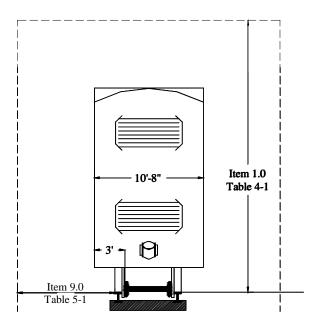
FIGURE 4-3: SIMPLIFIED CLEARANCE ENVELOPE
