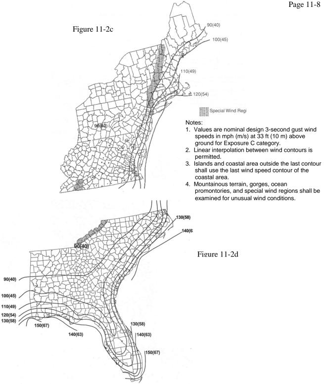
FIGURES 11-2c & -2d: BASIC WIND SPEED IN MILES PER HOUR AT 33 FT. ABOVE GROUND
