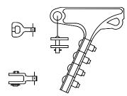
FIGURE 15-4a: TYPICAL BOLTED DEADEND CLAMP
