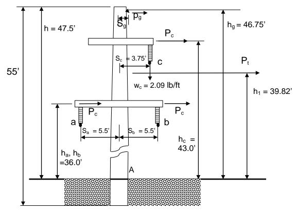
Figure 13-5: TS Type Structure Example
