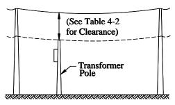
FIGURE 16-3: USE OF A SEPARATE POLE TO MOUNT A DISTRIBUTION TRANSFORMER
