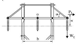
FIGURE 13-16: POLE TOP ASSEMBLY WITH TWO OUTSIDE BRACES
