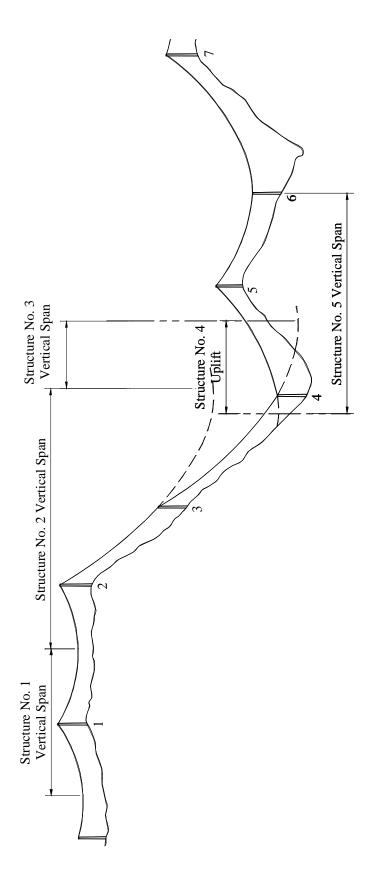
Figure 10-6 Sag Low Point, Vertical Spans and Uplift
