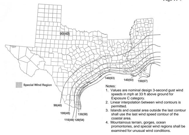
FIGURE 11-2e: BASIC WIND SPEED IN MILES PER HOUR AT 33 FT. ABOVE GROUND For use in calculating Extreme Wind Load. (50-year mean recurrence interval)
