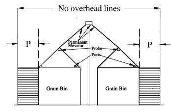
FIGURE 5-5: HORIZONTAL CLEARANCE TO GRAIN BINS, CONDUCTORS DISPLACED BY 6 PSF WIND
