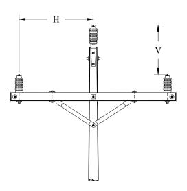
FIGURE 6-1: EXAMPLE OF VERTICAL AND HORIZONTAL SEPARATION VALUES
