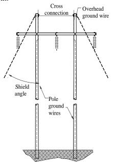
FIGURE 8-4: SHIELDING ANGLE, POLE AND OVERHEAD GROUND WIRES
