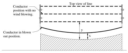
x = clearance from wind-displaced conductor, y= total horizontal clearance from conductor at rest
