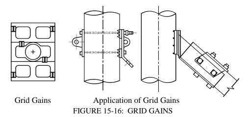
The gain plate (between a pole and a crossarm) and the reinforcing plate (on the outside of an arm) provide additional metal bearing surface for transfer of the vertical load from the crossarm to the crossarm mounting bolt. The gain plate eliminates a potential decay area between two wood contact areas. A reinforcing plate, also called a ribbed tie plate, will prevent the crossarm from splitting or checking when the nut is tightened.
