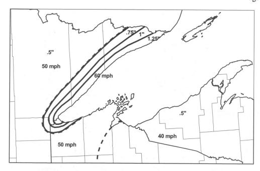
FIGURE 11-3d: UNIFORM ICE THICKNESS DUE TO FREEZING RAIN WITH CONCURRENT 3-SECOND GUST WIND SPEEDS FOR LAKE SUPERIOR (50 yr. mean recurrence)
