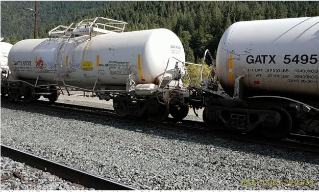
Residue Acid Tank cars - Hazardous Materials - Re-railed and moved to Dunsmuir Yard - Minor damage - No release.
